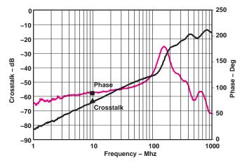
Phase at 10 MHz, -90.4 Degrees Crosstalk at 10 MHz, -63.9 dB
