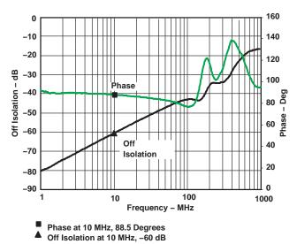
Figure 3. Off Isolation vs Frequency
